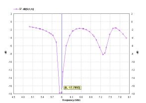
**Fig: 6.** Return Loss of the Proposed Rectangular Microstrip Patch Antenna with C inside C shaped slots
