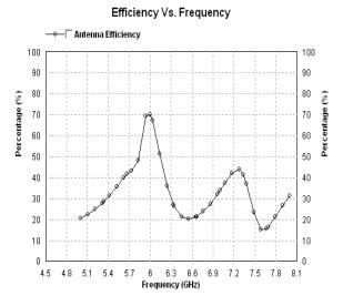
**Fig: 10.** Antenna efficiency & frequency of Rectangular Micro-strip Patch Antenna with C inside C shaped slots
