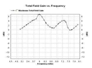
Fig: 7. Total field gain & frequency of Rectangular Micro-strip Patch Antenna with C inside C shaped slots
