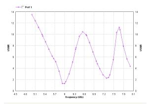
Fig: 3. VSWR of the Proposed Rectangular Microstrip Patch Antenna with C inside C shaped slots
