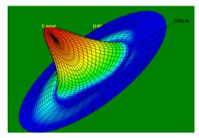
Fig: 4. Radiation pattern in 3D of the Proposed Rectangular Micro-strip Patch Antenna with C inside C shaped slots
