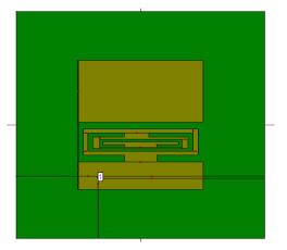
**Fig: 2.** Proposed Rectangular Micro-strip Patch Antenna with C inside C shaped slots feed at (-5, -8) point
