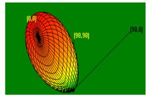
Fig: 12. 3D radiation pattern for 6 GHz frequency of Rectangular Micro-strip Patch Antenna with C inside C shaped slots
