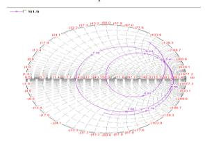
Fig: 5. Smith chart of the Proposed Rectangular Micro-strip Patch Antenna with C inside C shaped slots
