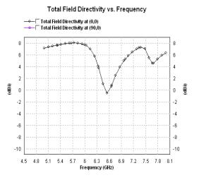
Fig: 8. Total field directivity & frequency of Rectangular Micro-strip Patch Antenna with C inside C shaped slots
