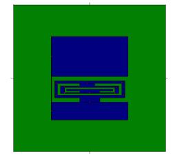
Fig: 1. Proposed Rectangular Micro-strip Patch Antenna with C inside C shaped slots
