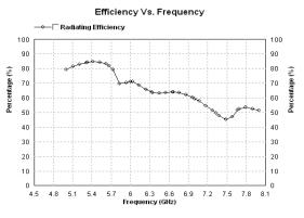
Fig: 11. Radiating efficiency & frequency of Rectangular Micro-strip Patch Antenna with C inside C shaped slots
